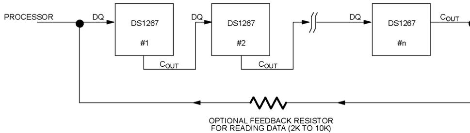
The C<sub>OUT</sub> output of the DS1267 can be used to drive the DQ input of another DS1267. When connecting multiple devices, the total number of bits transmitted is always 17 times the number of DS1267s in the daisy chain.
