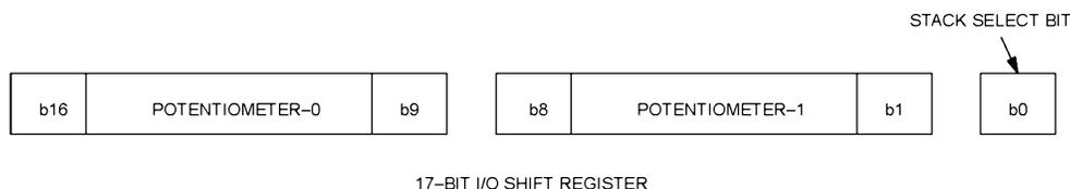
Transmission of data always begins with the stack select bit followed by the potentiometer-1 wiper position value and lastly the potentiometer-0 wiper position value.
