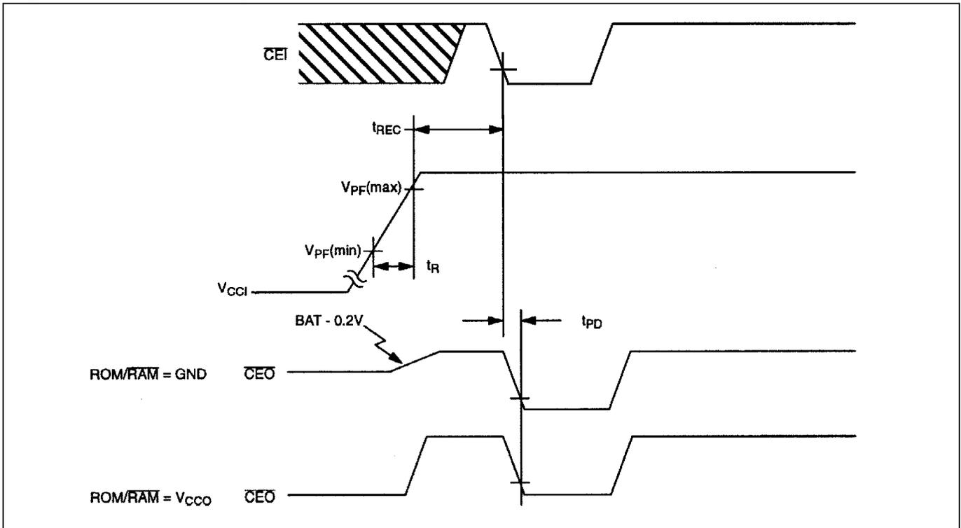
Figure 12. 5V Power-Down Condition
