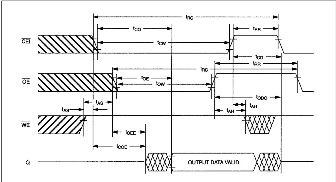
Figure 9. Timing Diagram: Write Cycle to Time Chip ROM/RAM =  $V_{CC0}$
