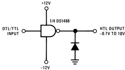
Figure 6. DTL/TTL-to-RTL Translator
