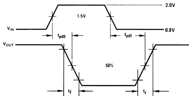
t<sub>r</sub> and t<sub>f</sub> are measured between 10% and 90% of the output waveform.
