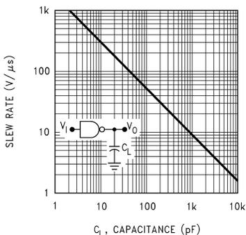
**Figure 9. Output Slew Rate vs Load Capacitance**
