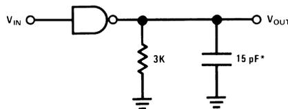
\*C<sub>L</sub> includes probe and jig capacitance.
