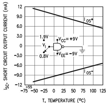
**Figure 8. Short-Circuit Output Current vs Temperature**
