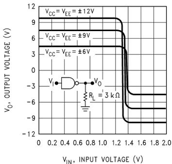
**Figure 7. Transfer Characteristics vs Power Supply Voltage**
