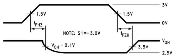
Figure 7. Receiver TRI-STATE Timing ( $t_{PHZ}$ ,  $t_{PZH}$ )
