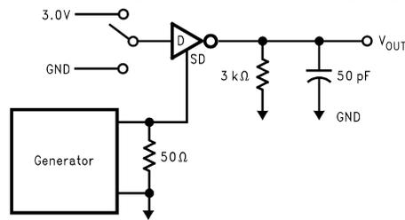
Driver Shutdown (SD) Delay Test Circuit
