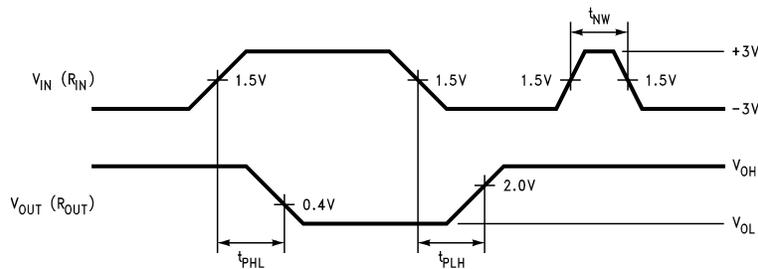
Figure 5. Receiver Propagation Delays and Noise Rejection
