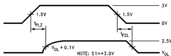
Figure 8. Receiver TRI-STATE Timing ( $t_{PLZ}$ ,  $t_{PZL}$ )
