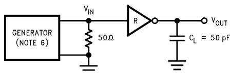
Figure 4. Receiver Propagation Delay Test Circuit
