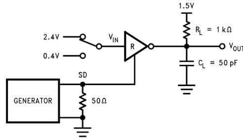
**Figure 8. Receiver SHUTDOWN (SD) Delay Test Circuit**
