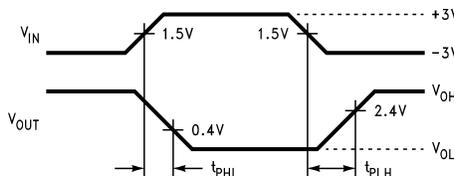
Figure 5. Receiver Propagation Delay Timing
