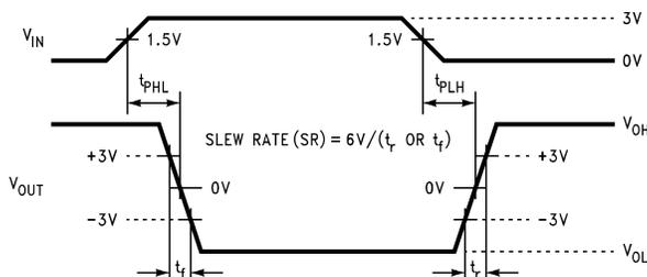
Figure 3. Driver Propagation Delay and Slew Rate Timing
