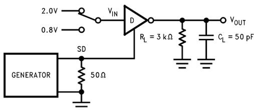
Figure 6. Driver SHUTDOWN (SD) Delay Test Circuit
