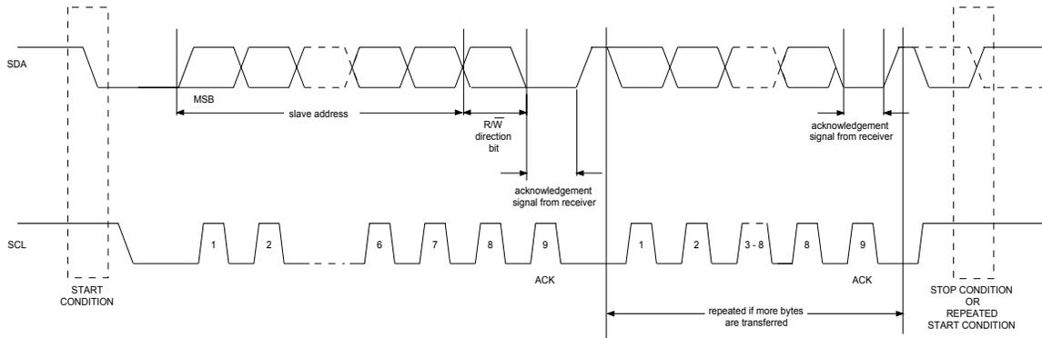
**Figure 7. Data Write: Slave Receiver Mode**
