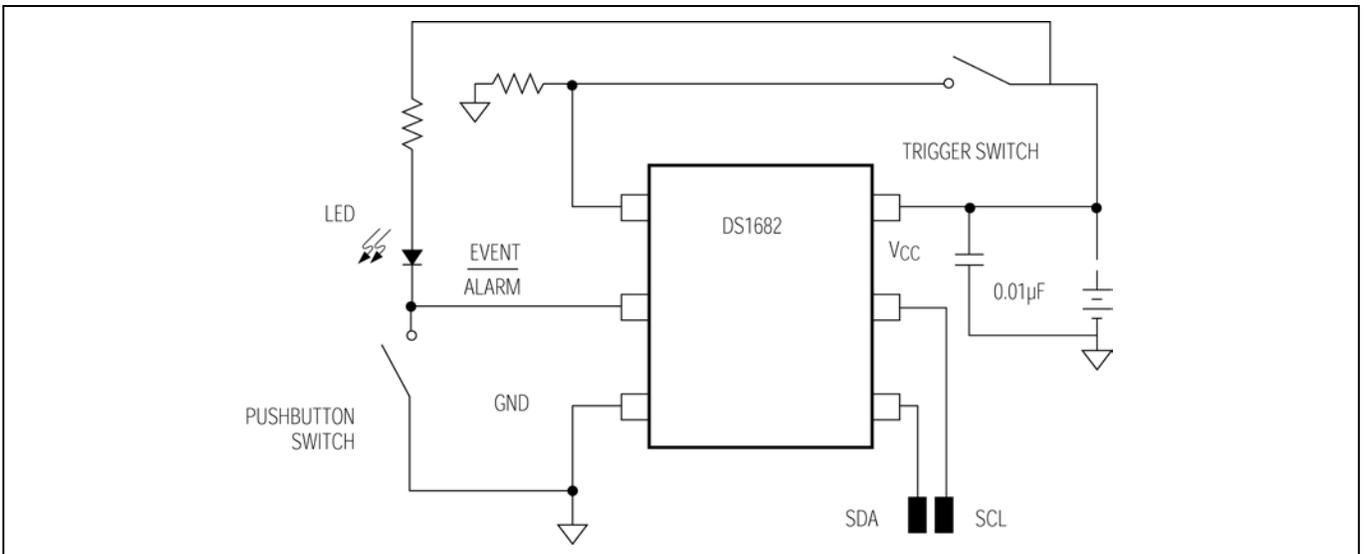
Figure 3 shows the DS1682 in a total time-of-use application where power may be removed at the same time as the end of the event. The  $V_{CC}$  slew rate at power-down is fast with respect to  $t_{EW}$ . A capacitor maintains  $V_{CC}$  on the DS1682 above 2.5V until the EEPROM write completes. A Schottky diode blocks current from the capacitor to other devices connected to  $V_{CC}$ .
