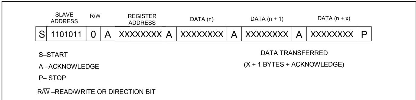
**Figure 9. Data Read—Slave Transmitter Mode**
