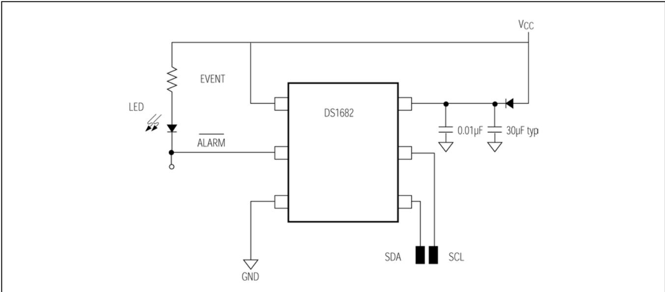
**Figure 4. Total Time-of-Use Application with Slow  $V_{CC}$  Slew Rate**
