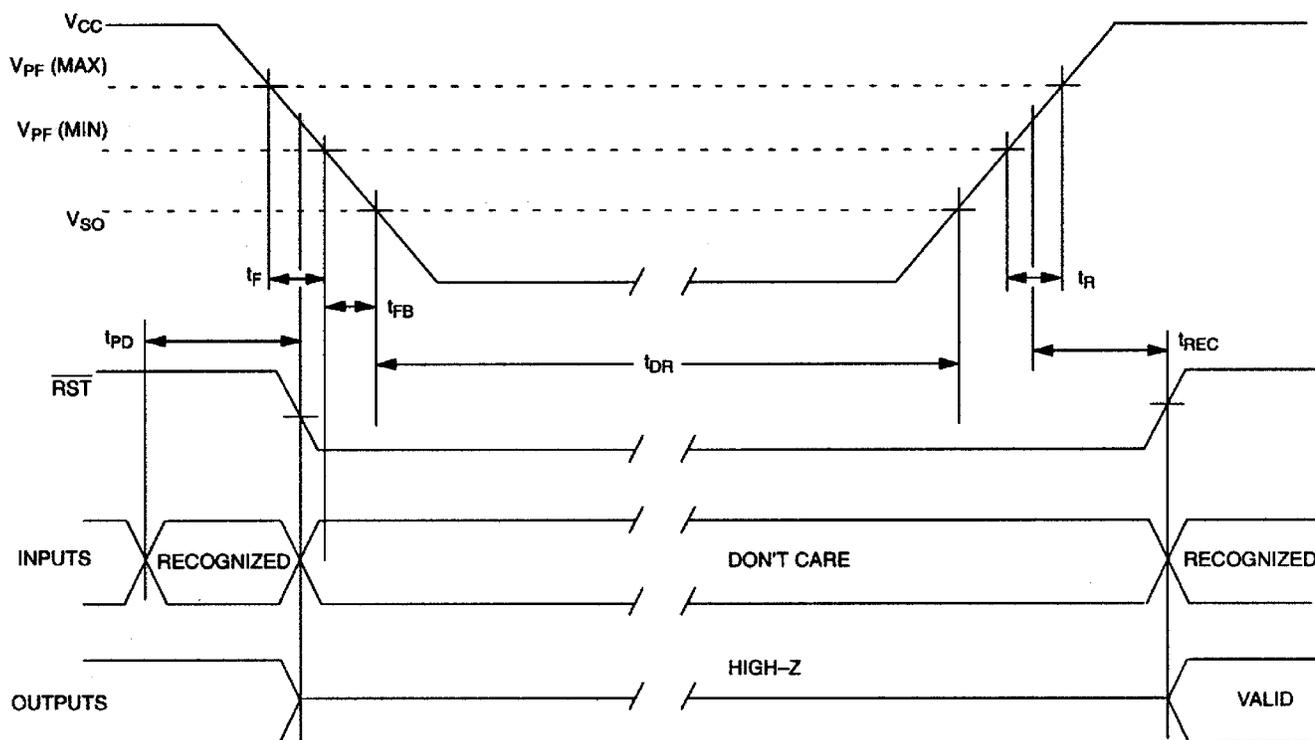
**POWER-UP/DOWN CHARACTERISTICS** $(V_{CC} = 3.3V \pm 10\%$ , Over the operating range)
