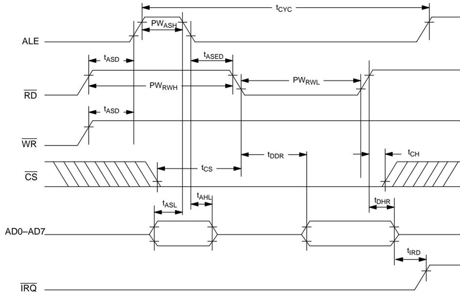
**RTC AC TIMING CHARACTERISTICS**(0°C to 70°C;  $V_{CC} = 5.0V \pm 10\%$ )
