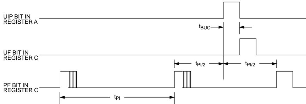
$t_{PI}$  = PERIODIC INTERRUPT TIME INTERNAL PER TABLE 1
