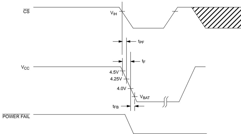
**POWER-UP POWER-DOWN TIMING 5 VOLT DEVICE** $(t_A = 25^\circ\text{C})$
