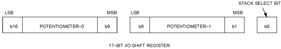
Transmission of data always begins with the stack select bit followed by the potentiometer-1 wiper position value and lastly the potentiometer-0 wiper position value (see Figure 2(a)).
