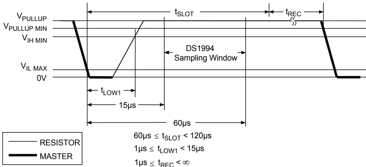
**Figure 11. READ/WRITE TIMING DIAGRAM (continued)****Write-Zero Time Slot**
