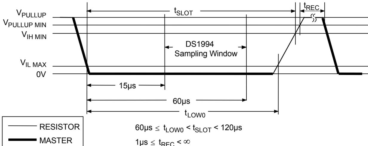
**Read-Data Time Slot**
