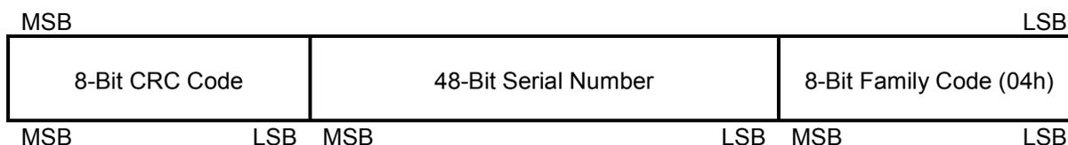
**Figure 3. 1-WIRE CRC CODE**
