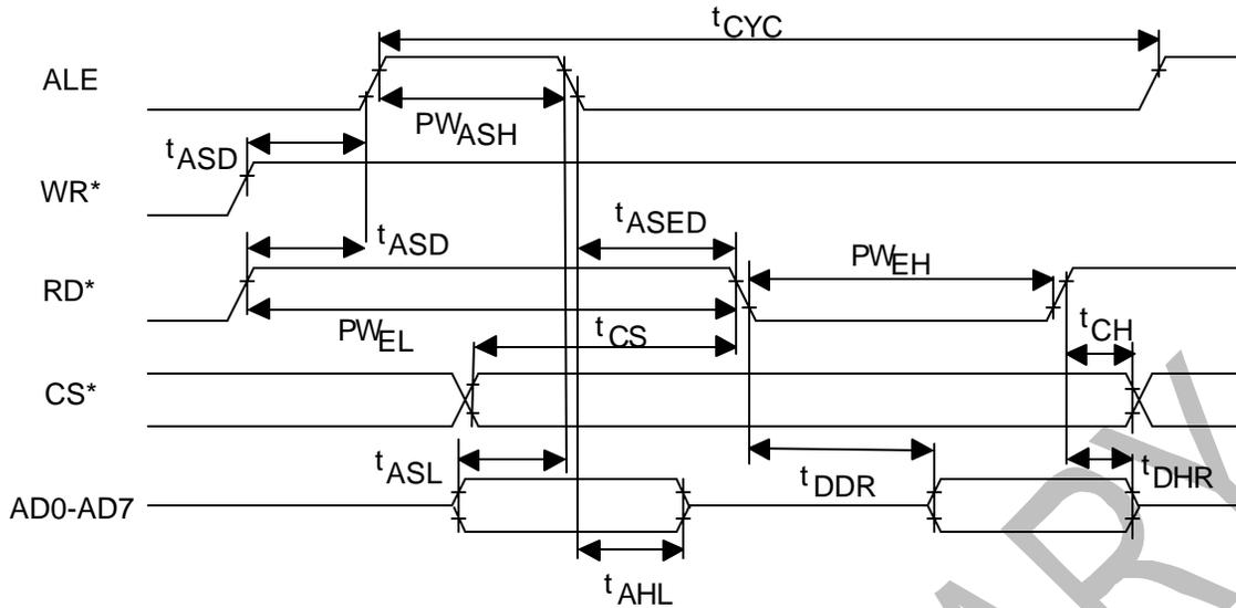
**INTEL BUS WRITE TIMING (BTS = 0 / MUX = 1) Figure 37-2**
