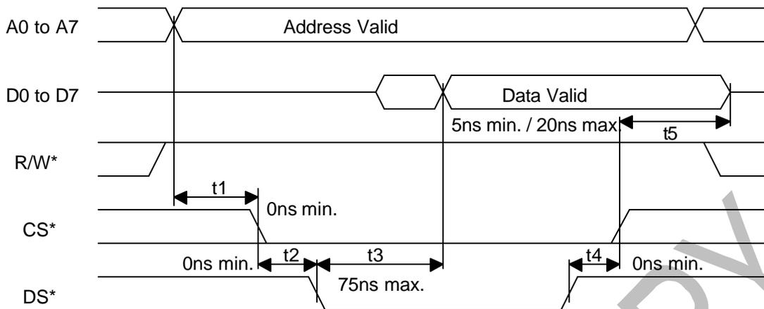
**MOTOROLA BUS WRITE TIMING (BTS = 1 / MUX = 0) Figure 37-7**
