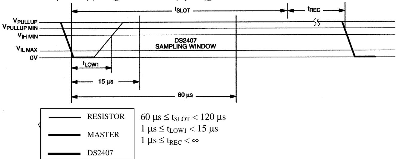
**READ/WRITE TIMING DIAGRAM Figure 15 (cont'd)****Write-0 Time Slot**
