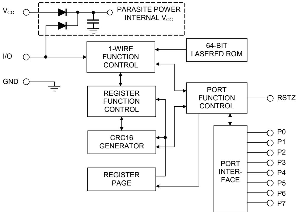
**Figure 2. HIERARCHICAL STRUCTURE FOR 1-Wire PROTOCOL**
