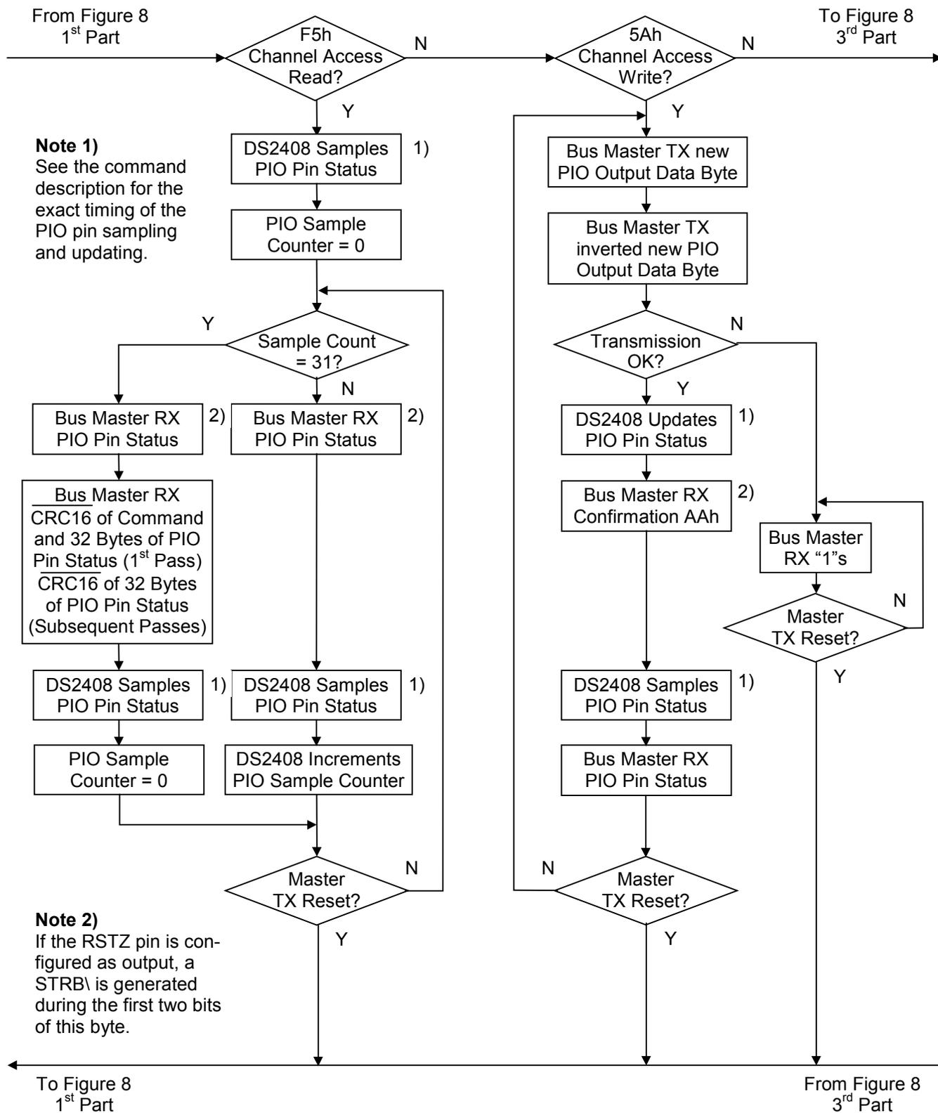
**Figure 8-3. CONTROL FUNCTIONS FLOW CHART**
