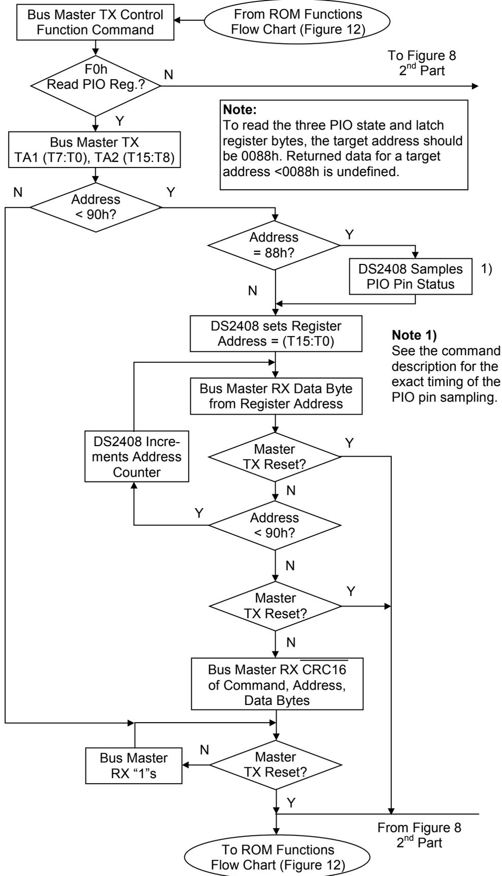
**Figure 8-2. CONTROL FUNCTIONS FLOW CHART**
