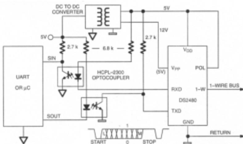
The circuit in Figure 10d is essentially the same as in Figure 10a. The main difference is the opto-isolation. The characteristics of the opto-isolators are not very critical. Using a different type will affect the values of the resistors that limit the current through the LEDs and bias the photo transistors.
