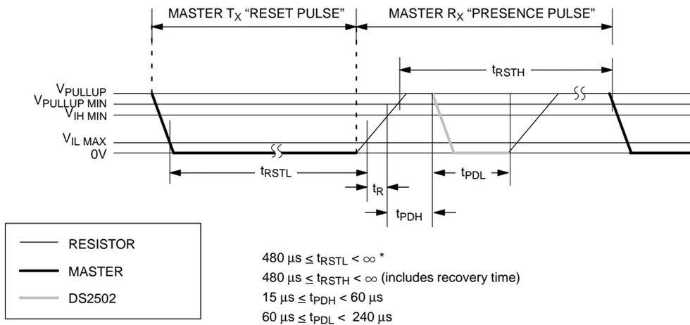
\* In order not to mask interrupt signaling by other devices on the 1-Wire bus,  $t_{RSTL} + t_R$  should always be less than  $960 \mu\text{s}$ .
