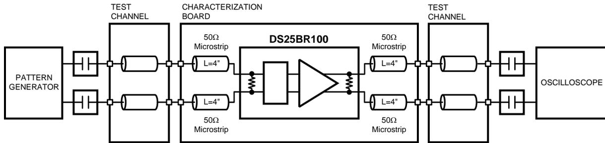
**Figure 5. Pre-emphasis and Equalization Performance Test Circuit**
