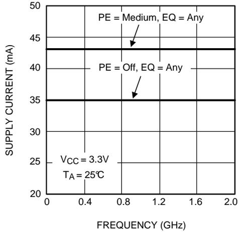
Figure 20. Power Supply Current as a Function of Frequency
