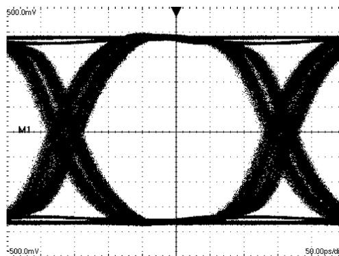
Figure 20. An Equalized 3.125 Gbps NRZ PRBS-7 After 70" Differential FR-4 Stripline
