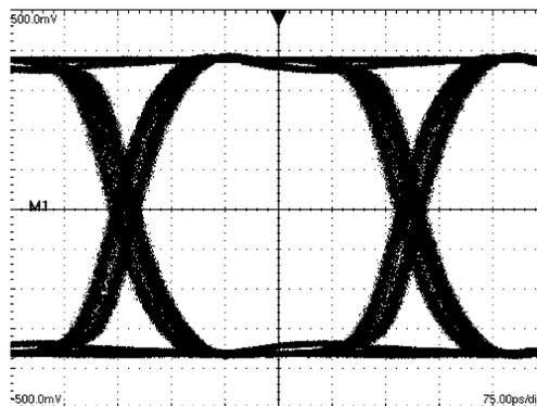
Figure 18. An Equalized 2.5 Gbps NRZ PRBS-7 After 70" Differential FR-4 Stripline
