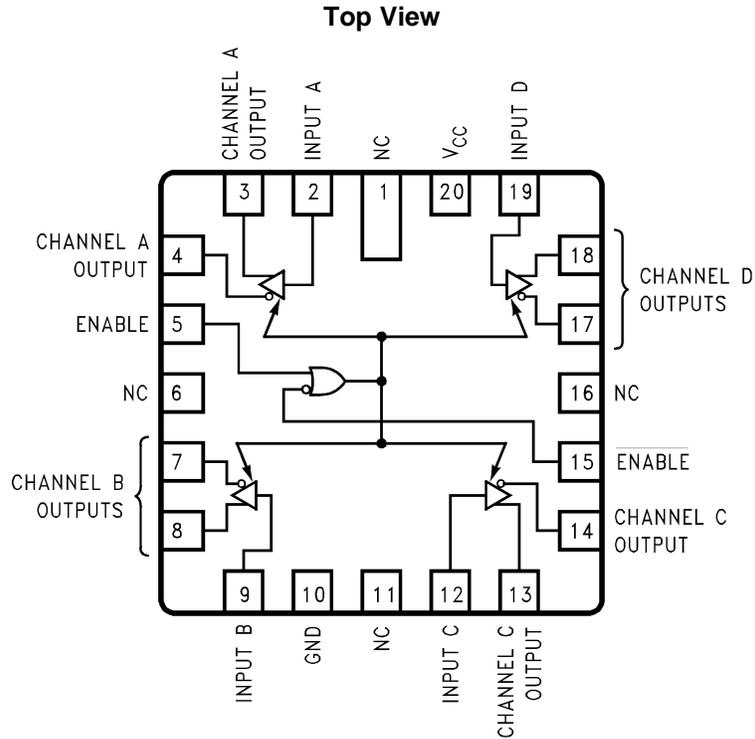
**Figure 2. 20-Lead LCCC Package
