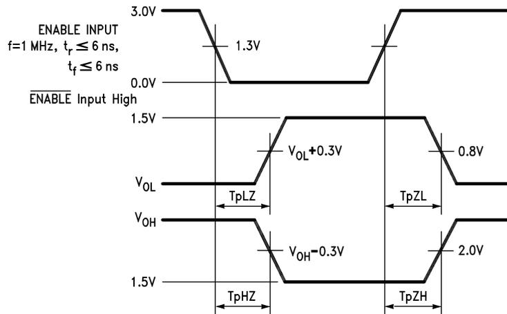
Figure 28. Enable and Disable Times
