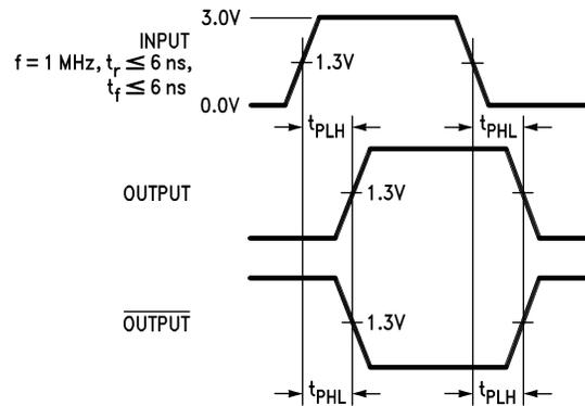
Figure 27. Propagation Delays
