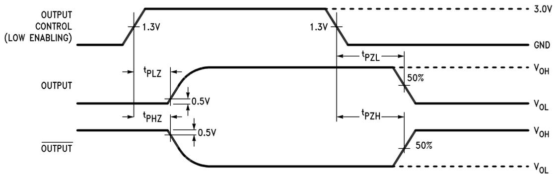
Figure 20. TRI-STATE Output Enable and Disable Waveforms
