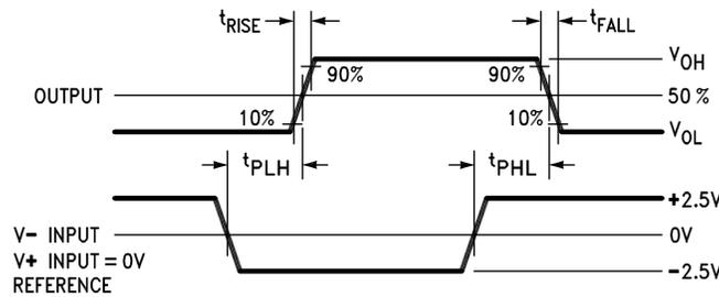
Figure 19. Propagation Delay
