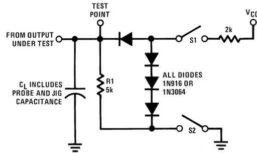
**Figure 3. Load Test Circuit for TRI-STATE Outputs**
