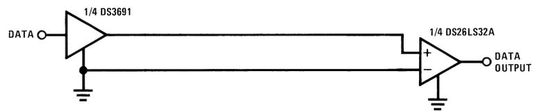
Figure 7. Single Wire with Driver Ground Reference—RS-423
