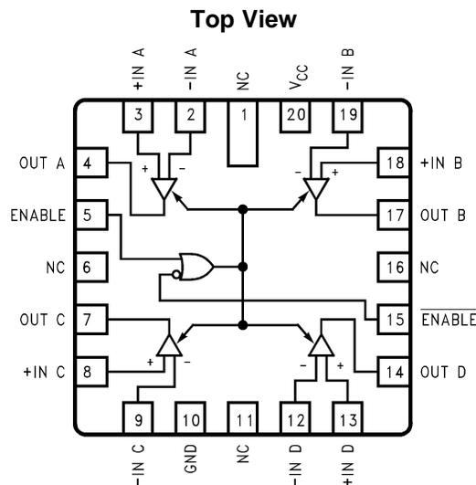
Figure 2. 20-Lead LCCC Package
