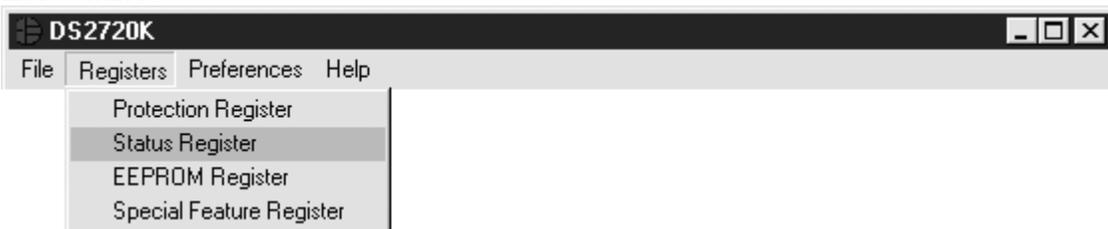
The Registers Menu gives immediate access to the status and function registers of the DS2720. Selecting any of the registers will open an individual control window giving the user a description of each register bit and the ability to read or write it. See the protection register window example.
