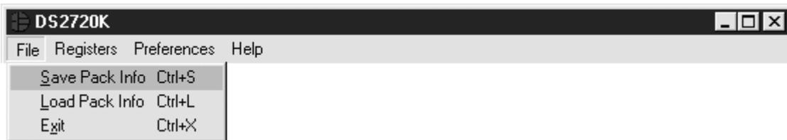
The File Menu allows the user to store information from a file directly into the Device Setup and Battery Data sections under the Pack Info Tab or take the same Pack Information and store to a file. These functions do not directly write or read the DS2720. It is still necessary for the user to store or recall this information to or from the device by issuing a WRITE or READ command under the Pack Info Tab.
