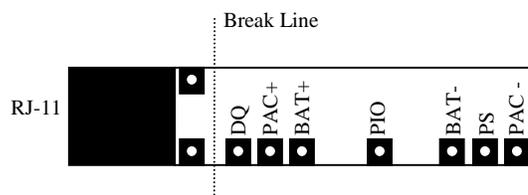
Figure 1: Communication Connections
