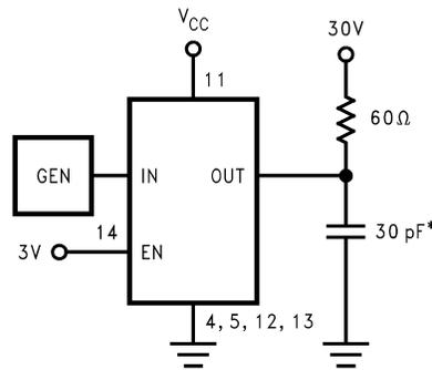
\*Includes probe and jig capacitance.
