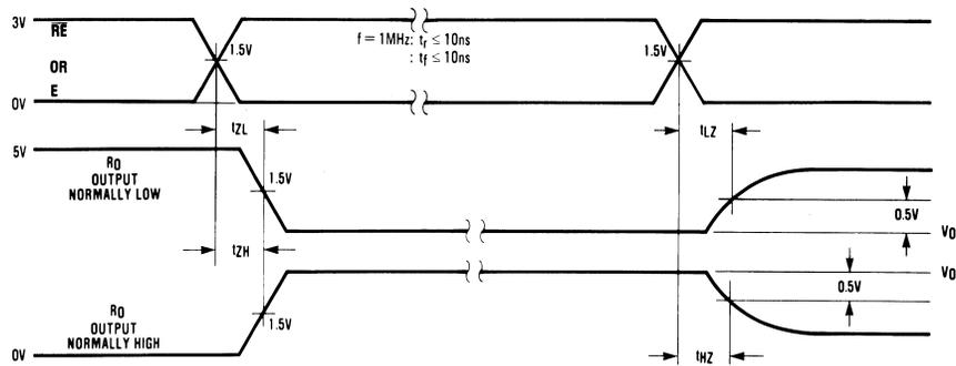
Figure 7. Receiver Enable/Disable Propagation Delay Timing
