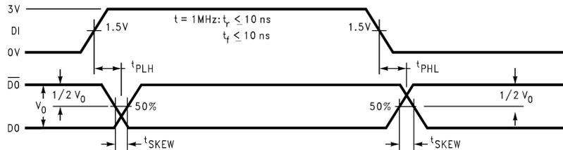
Note:  $t_{PLH}$  and  $t_{PHL}$  are measured to the respective 50% points.  $t_{SKEW}$  is the difference between propagation delays of the complementary outputs.
