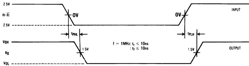
Note: Differential input voltage may be realized by grounding  $\overline{RI}$  and pulsing  $RI$  between +2.5V and -2.5V.
