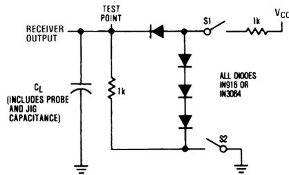
Figure 5. Receiver Propagation Delay Test Circuit
