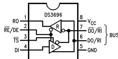
**Figure 2. PDIP (Top View)**
