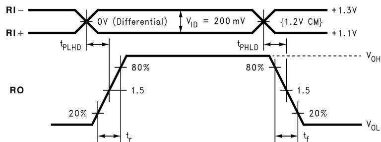
Figure 9. Receiver Propagation Delay and Transition Time Waveforms
