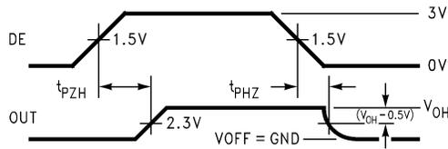
Figure 9. TRI-STATE Waveforms ( $t_{PZH}$ ,  $t_{PHZ}$ )
