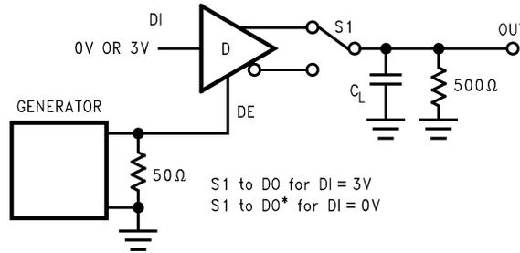
Figure 8. TRI-STATE Test Circuit ( $t_{PZH}$ ,  $t_{PHZ}$ )
