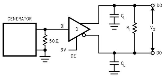
Figure 6. Driver Differential Propagation Delay Test Circuit
