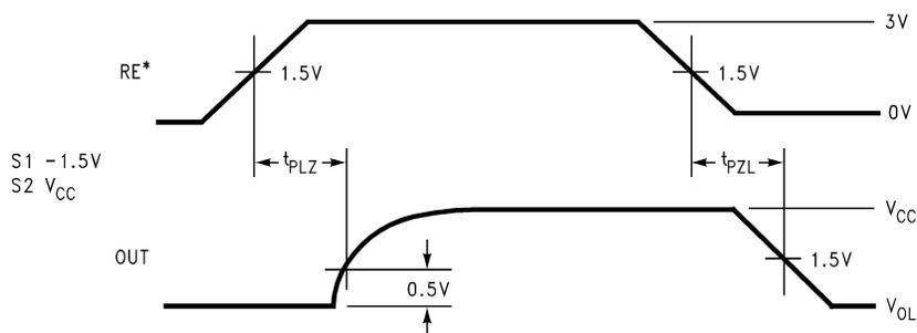
**Figure 16. Receiver Enable and Disable Waveforms ( $t_{PLZ}$ ,  $t_{PZL}$ )**
