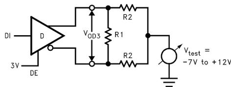
Figure 3. Driver  $V_{OD3}$
