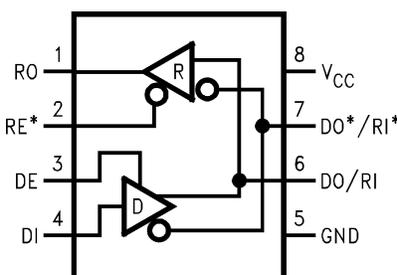
**Figure 1. 8-Pin PDIP or SOIC
