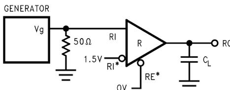
Figure 13. Receiver Differential Propagation Delay Test Circuit
