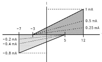
Figure 19. Input Current vs Input Voltage Operating Range
