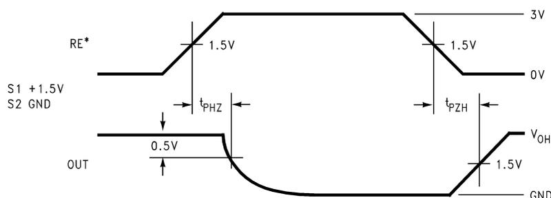
**Figure 17. Receiver Enable and Disable Waveforms ( $t_{PHZ}$ ,  $t_{PZH}$ )**
