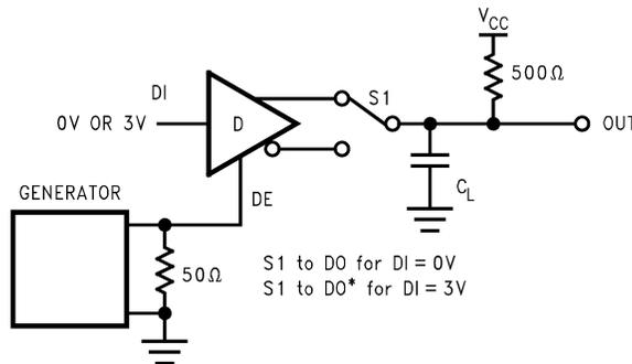
Figure 10. TRI-STATE Test Circuit ( $t_{PZL}$ ,  $t_{PLZ}$ )
