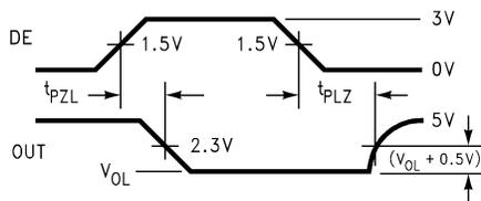
Figure 11. TRI-STATE Waveforms ( $t_{PZL}$ ,  $t_{PLZ}$ )
