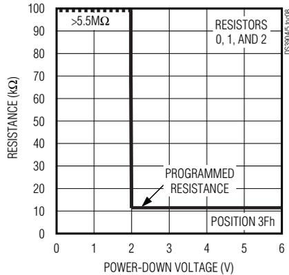
**POSITION 3Fh RESISTANCE vs. SUPPLY VOLTAGE**
