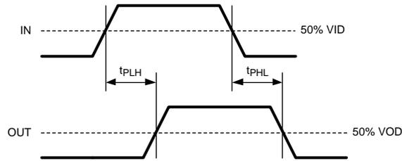
Figure 3. Propagation Delay from input to output
