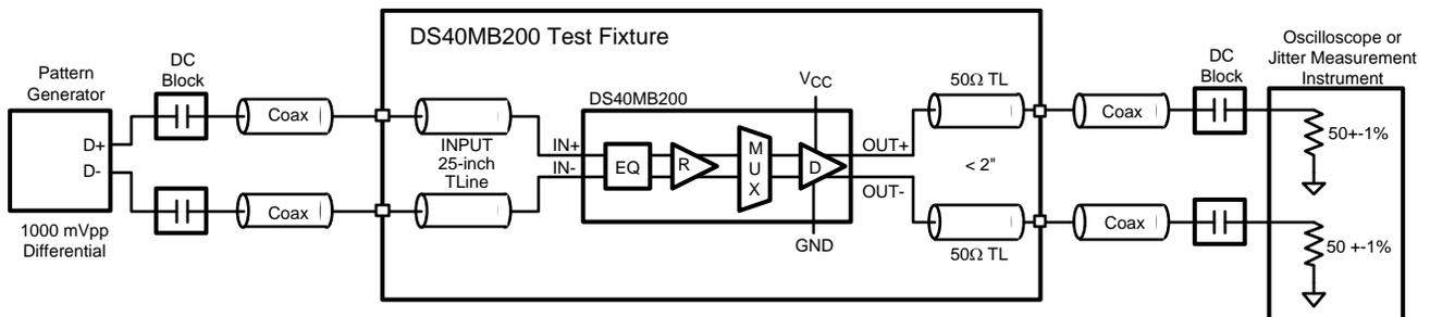
Figure 5. AC Test Circuit
