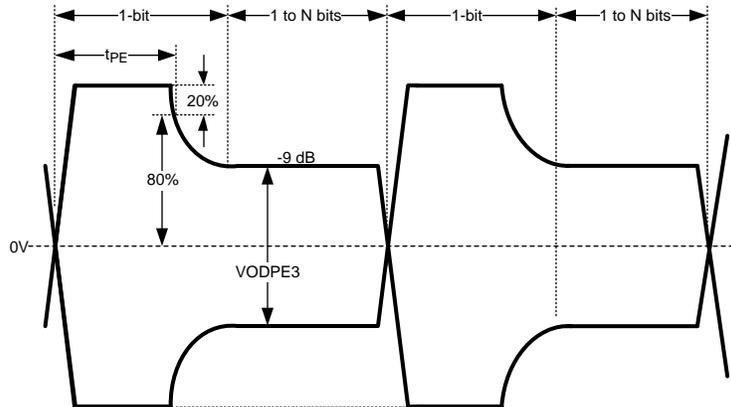
Figure 4. Test condition for output pre-emphasis duration
