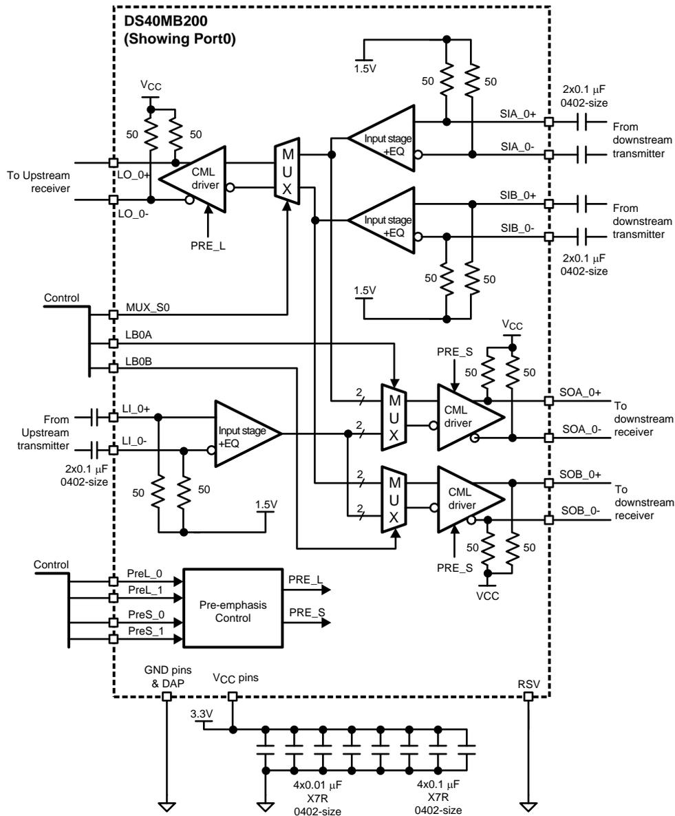
Figure 10. Application Diagram (showing data paths of port 0)
