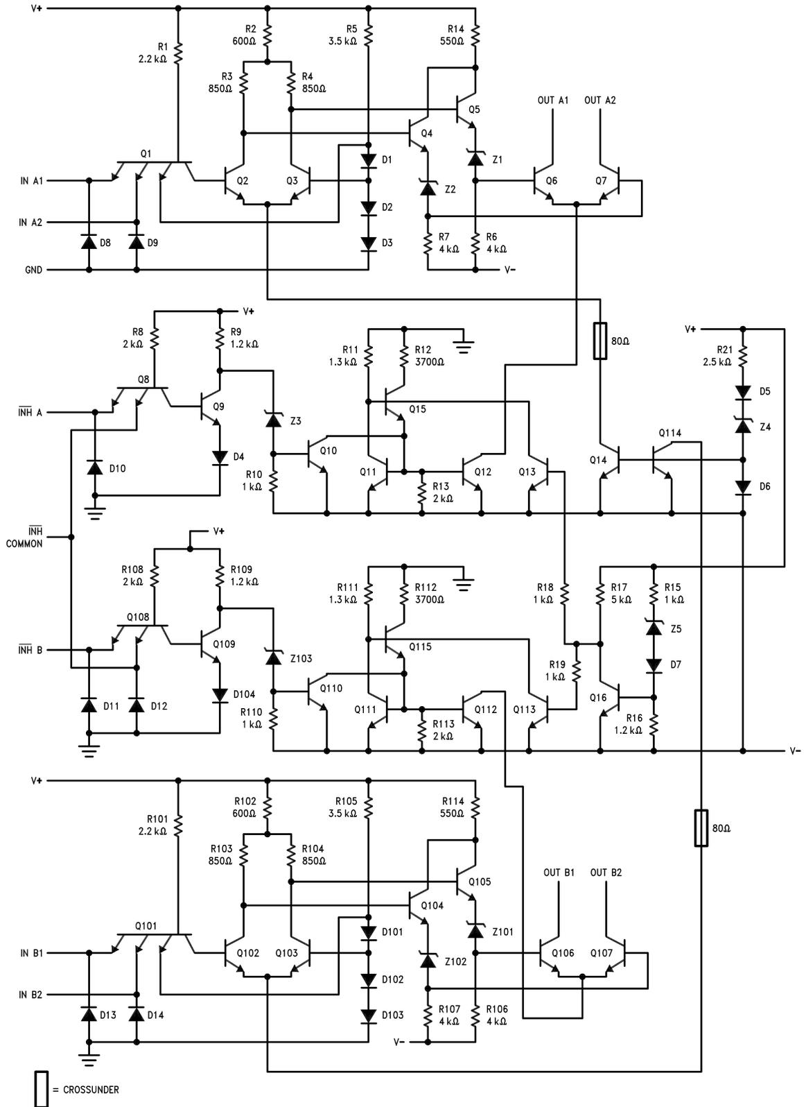
FIGURE 3. Equivalent Circuit
