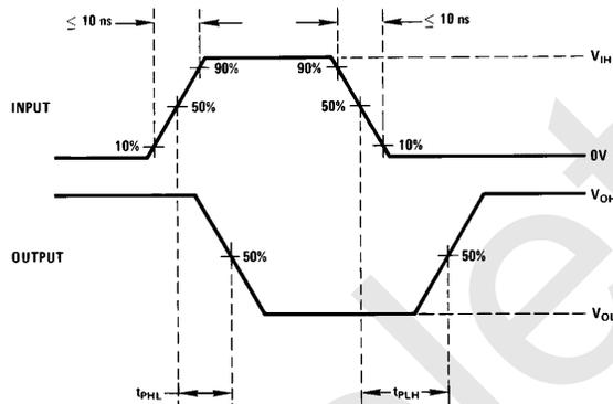
**Note 1:** The pulse generator has the following characteristics:  $Z_{OUT} = 50\Omega$ ,  $PRR = 100\text{ kHz}$ ,  $t_W = 1\ \mu\text{s}$ .
