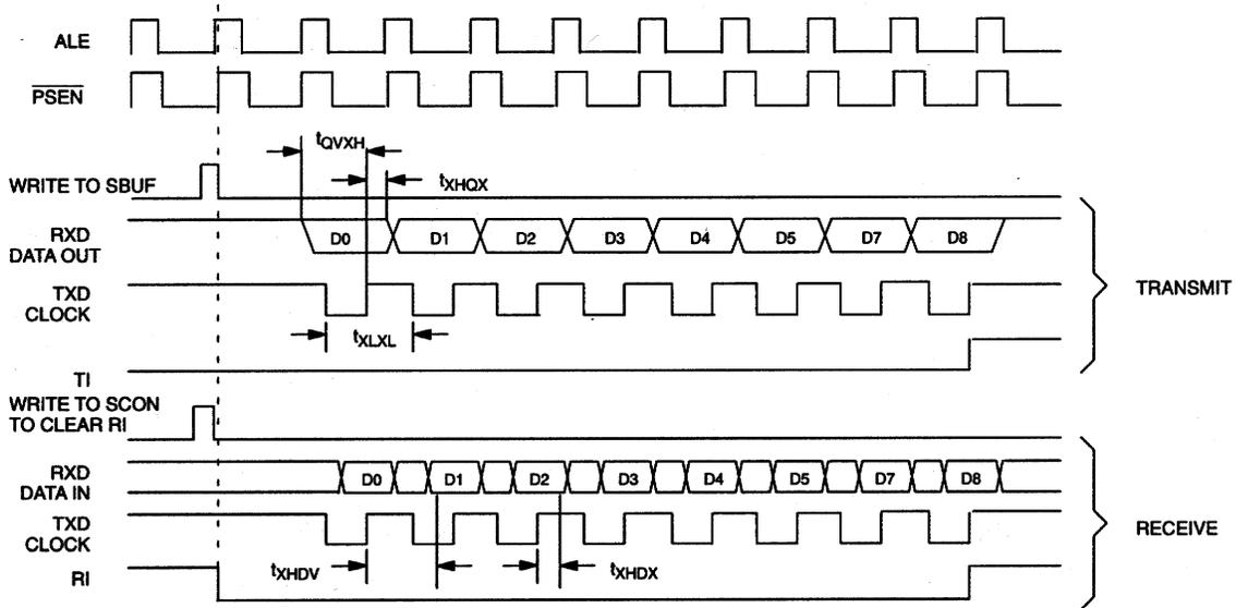
SERIAL PORT 0 (SYNCHRONOUS MODE)
