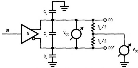
FIGURE 1.  $V_{OD}$  and  $V_{OC}$  Test Circuit
