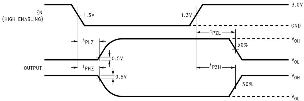
Figure 5. TRI-STATE Output Enable and Disable Waveforms
