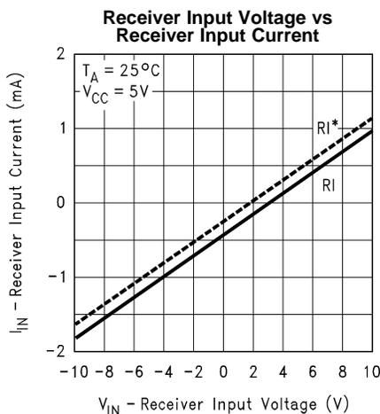
The DS89C386 is V.11 compatible.  $I_{IN}$  (RI input) is not  $\geq 0$  when  $V_{IN} = 3V$  due to internal failsafe bias resistors (see Figure 10). See ITU V.11 for complete conditions.
