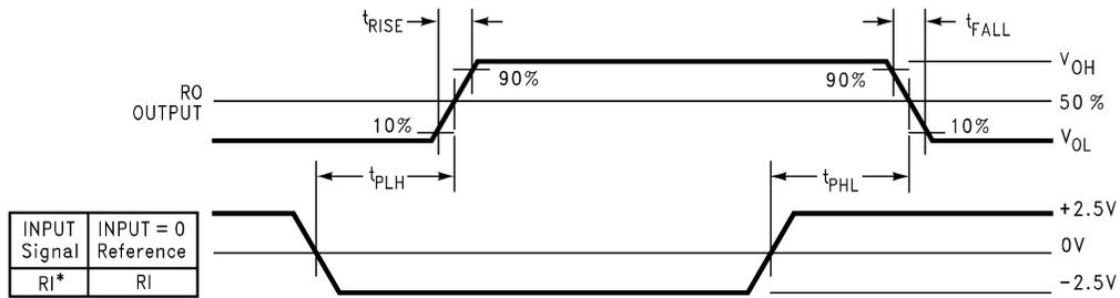
Figure 3. Propagation Delays
