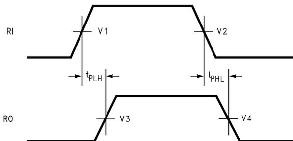
Figure 9. Waveforms for Circuit 1 – Propagation Delay Waveforms for Circuit 1 and Circuit 2
