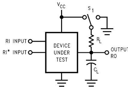
C<sub>L</sub> includes load and test jig capacitance.
