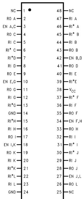
**Figure 1. 48-Pin SSOP**
