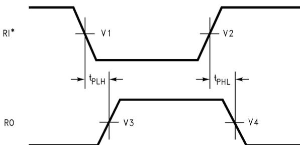
Figure 10. Waveforms for Circuit 2 – Propagation Delay Waveforms for Circuit 1 and Circuit 2
