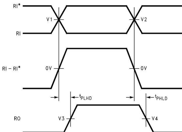
**Figure 12. Waveforms for Circuit 3 – Propagation Delay Waveforms**
