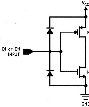
FIGURE 13. Driver Input or Driver Enable Equivalent Circuit
