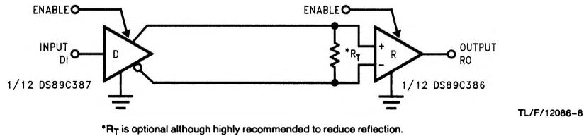
**FIGURE 5. Two-Wire Balanced System, RS-422**
