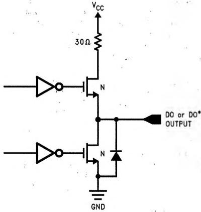
FIGURE 12. Driver Output Equivalent Circuit
