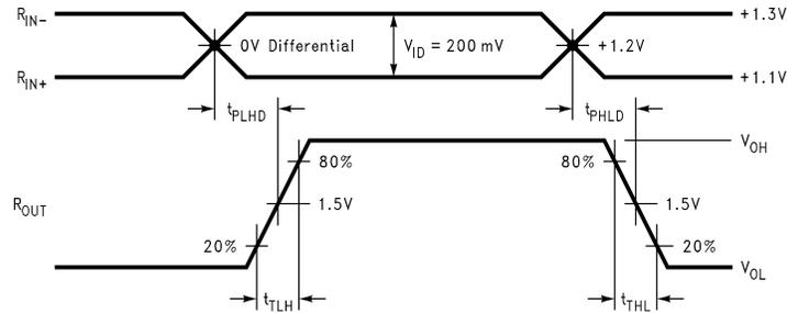
**Figure 4. Receiver Propagation Delay and Transition Time Waveforms**
