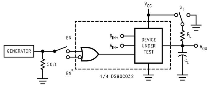
$C_L$  includes load and test jig capacitance.
