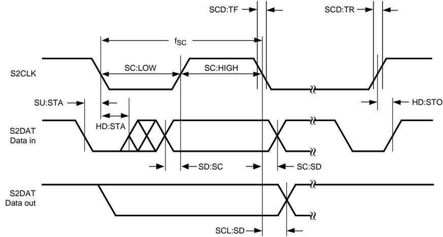
Figure 3. Two-Wire Serial Communication Interface Timing Diagram
