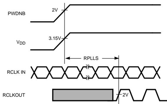
Figure 8. Receiver Phase Lock Loop Wake-up Time
