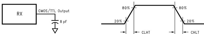
Figure 7. LVC MOS/LVTTL Output Load and Transition Times
