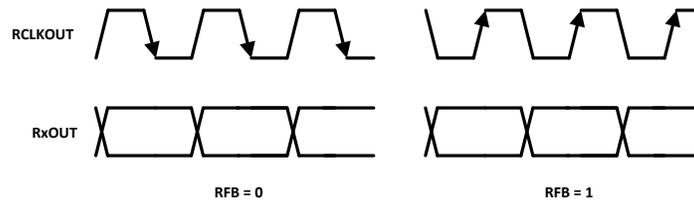
Figure 11. RFB: LVTTTL Level Programmable Strobe Select
