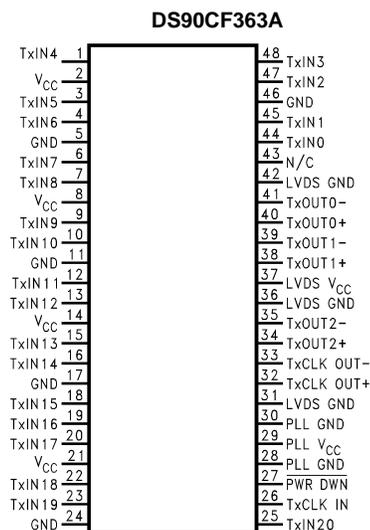
Figure 16. 48 Pin TSSOP - See Package Number DGG
