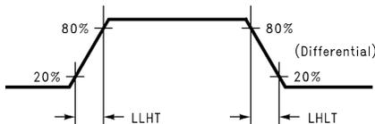
Figure 5. DS90C363A/DS90CF363A (Transmitter) LVDS Transition Times
