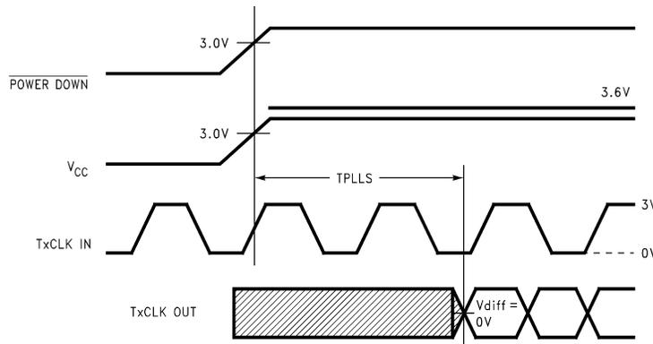
Figure 9. DS90C363A/DS90CF363A (Transmitter) Phase Lock Loop Set Time
