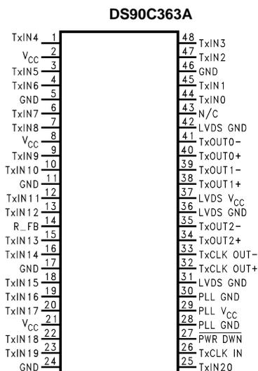
Figure 15. 48 Pin TSSOP - See Package Number DGG
