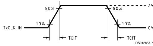
**FIGURE 5. DS90C383 (Transmitter) Input Clock Transition Time**
