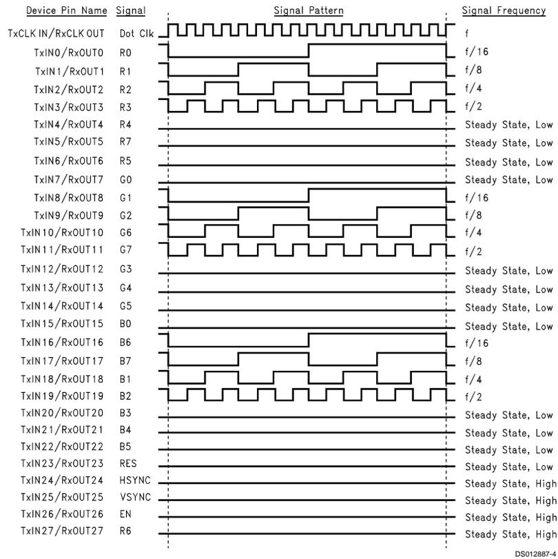
FIGURE 2. "16 Grayscale" Test Pattern (Notes 6, 7, 8, 9)
