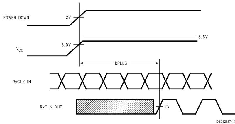
**FIGURE 12. DS90CF384 (Receiver) Phase Lock Loop Set Time**
