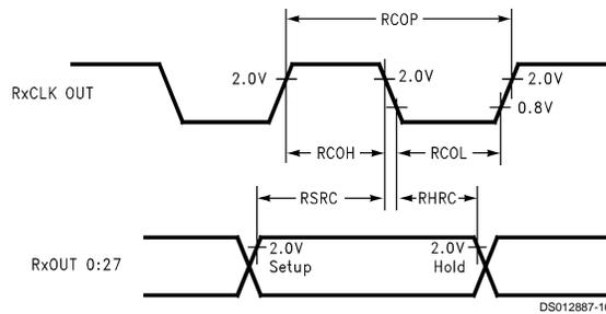
**FIGURE 8. DS90CF384 (Receiver) Setup/Hold and High/Low Times**
