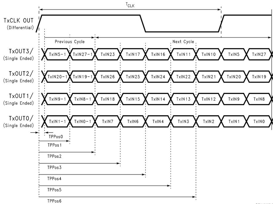
FIGURE 17. Transmitter LVDS Output Pulse Position Measurement
