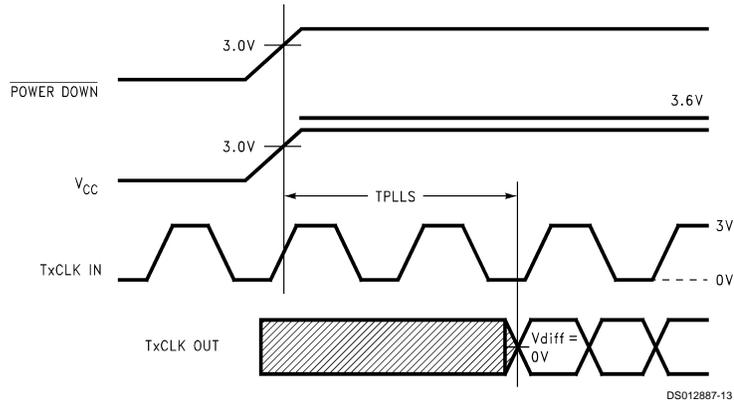
**FIGURE 11. DS90C383 (Transmitter) Phase Lock Loop Set Time**
