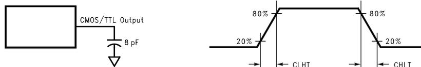
Figure 4. Receiver CMOS/TTL Output Load and Transition Times
