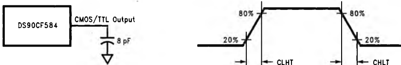
FIGURE 4. DS90CF584 (Receiver) CMOS/TTL Output Load and Transition Times
