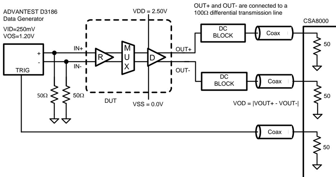
Figure 4. Differential Driver AC Test Circuit
