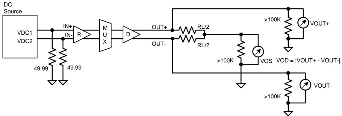
Figure 3. Differential Driver DC Test Circuit
