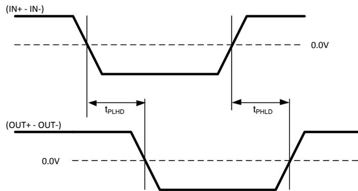
Figure 8. LVDS Output Propagation Delay
