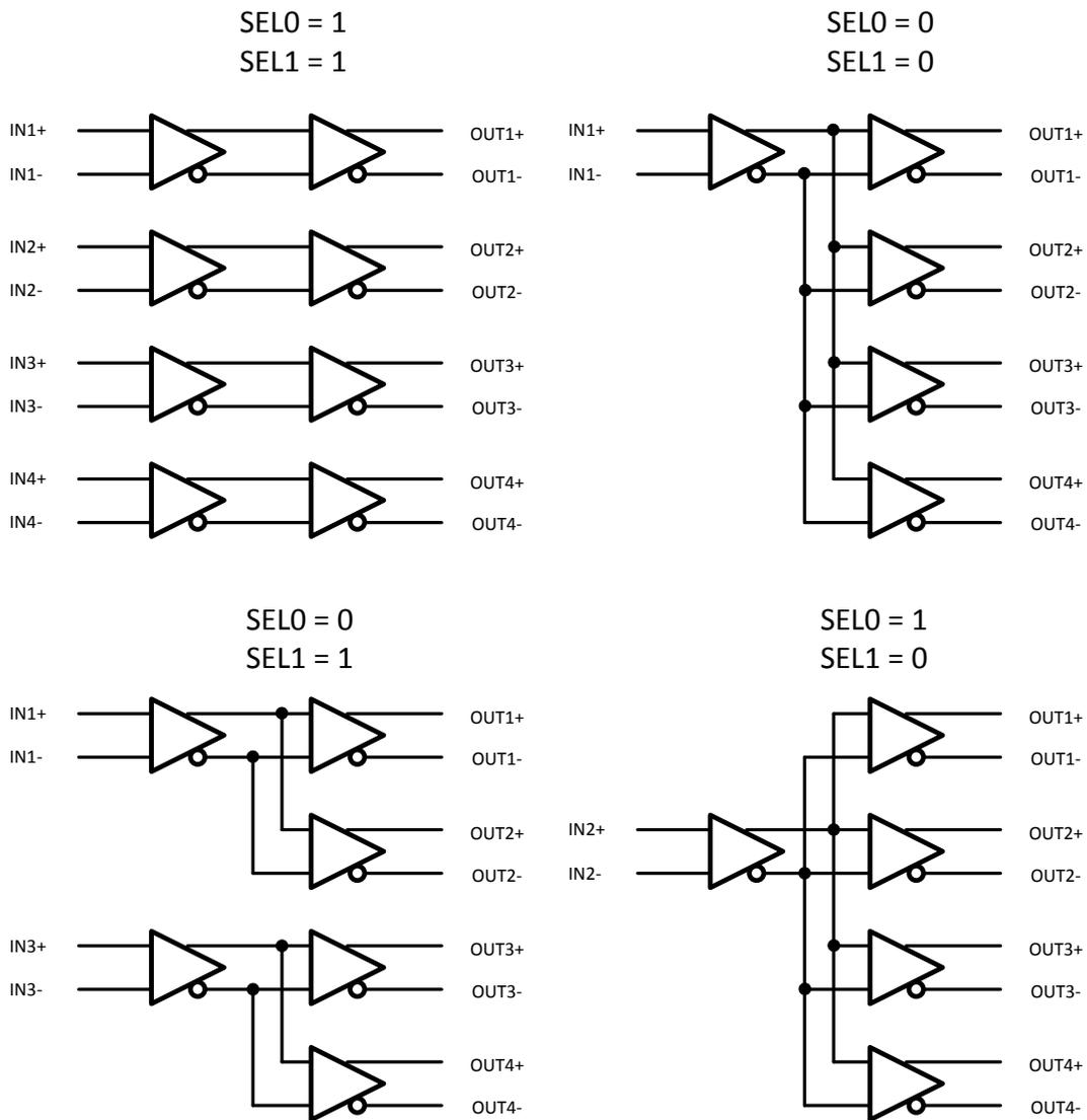
**Figure 2. DS90CP04 Configuration Select Decode**
