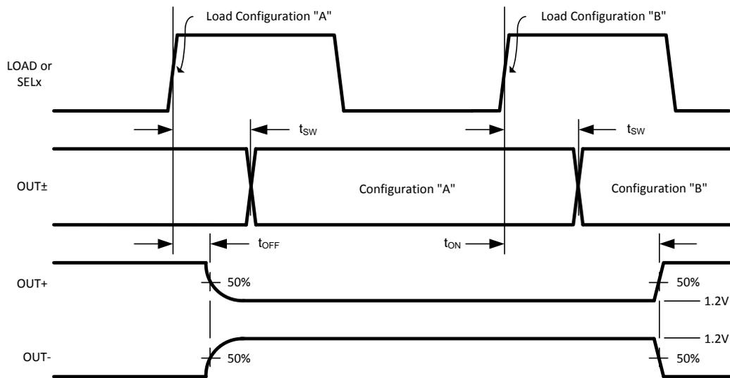
Figure 11. Configuration and Output Enable/Disable Timing
