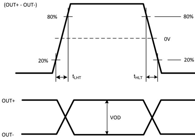
Figure 7. LVDS Output Transition Time
