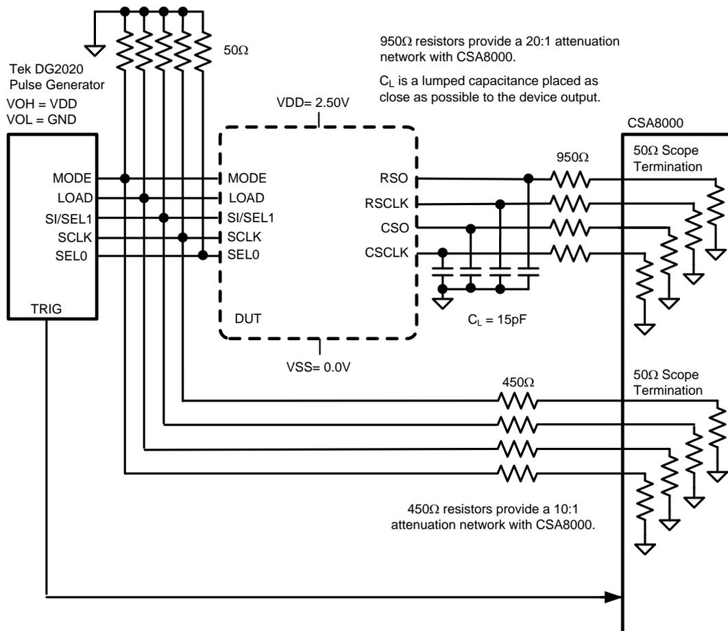
Figure 5. LVC MOS Driver AC Test Circuit <sup>(9)</sup>
