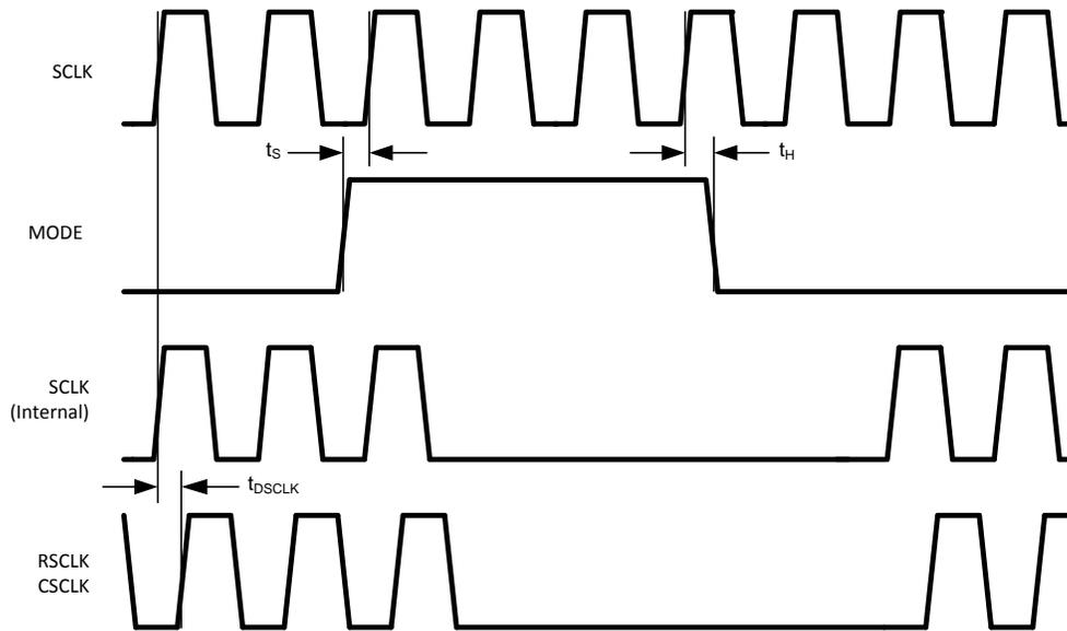
Figure 10. Serial Interface— MODE Timing and Functionality
