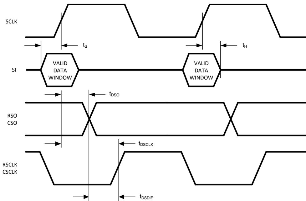
Figure 9. Serial Interface Propagation Delay and Input Timing Waveforms
