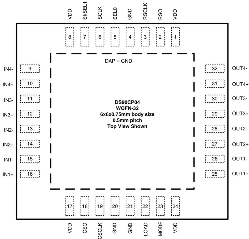
Figure 1. 32 Pin (Top View)
