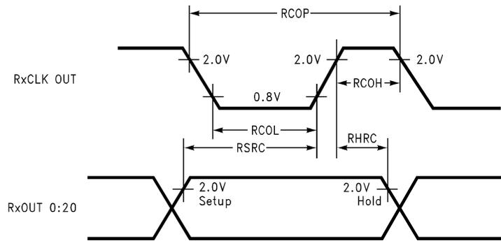
Figure 6. DS90CR218 (Receiver) Setup/Hold and High/Low Times
