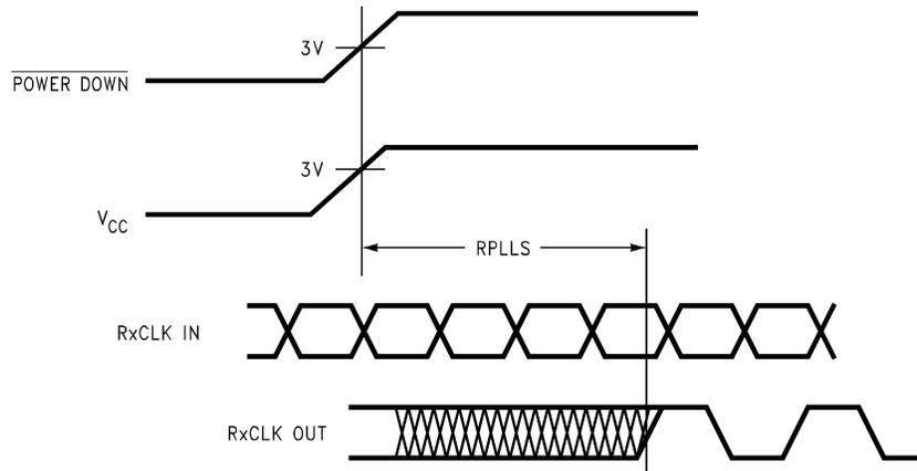
Figure 8. DS90CR218 (Receiver) Phase Lock Loop Set Time
