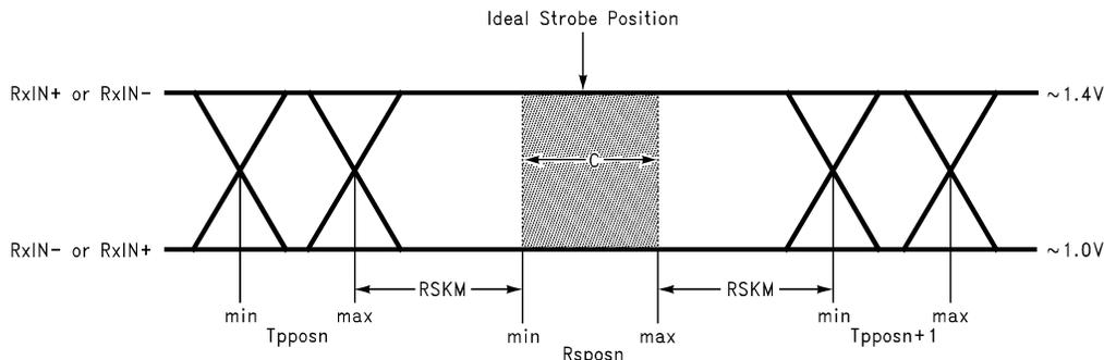
C—Setup and Hold Time (Internal data sampling window) defined by Rspesn (receiver input strobe position) min and max
