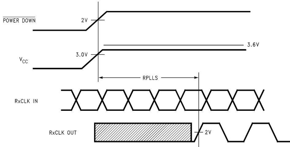
Figure 7. DS90CR286A/DS90CR216A (Receiver) Phase Lock Loop Set Time
