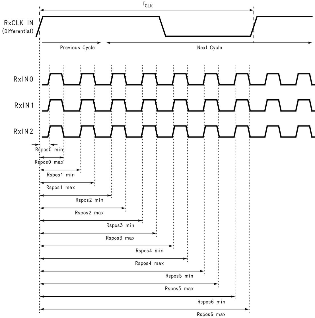
Figure 12. DS90CR216A (Receiver) LVDS Input Strobe Position
