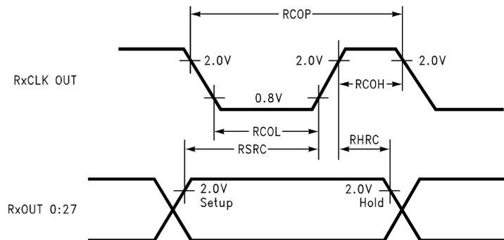
Figure 5. DS90CR286A/DS90CR216A (Receiver) Setup/Hold and High/Low Times
