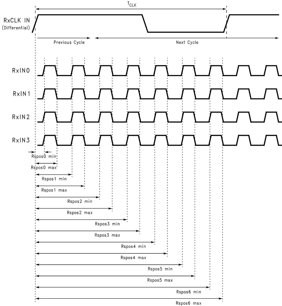
Figure 11. DS90CR286A (Receiver) LVDS Input Strobe Position
