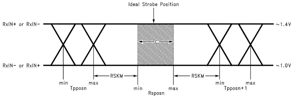
C—Setup and Hold Time (Internal data sampling window) defined by Rspostn (receiver input strobe position) min and max
