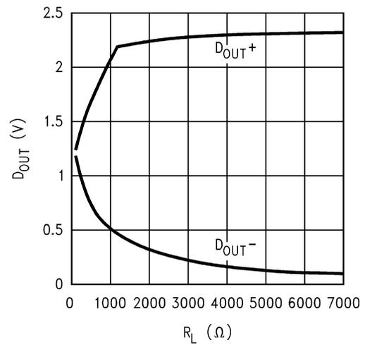
Figure 8. Typical DS90LV031,  $D_O$  vs  $R_L$ ,
