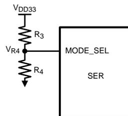
Figure 12. MODE\_SEL Connection Diagram
