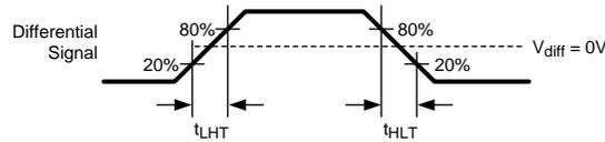
Figure 5. Serializer CML Output Load and Transition Time
