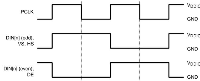
Figure 3. Checkboard Data Pattern
