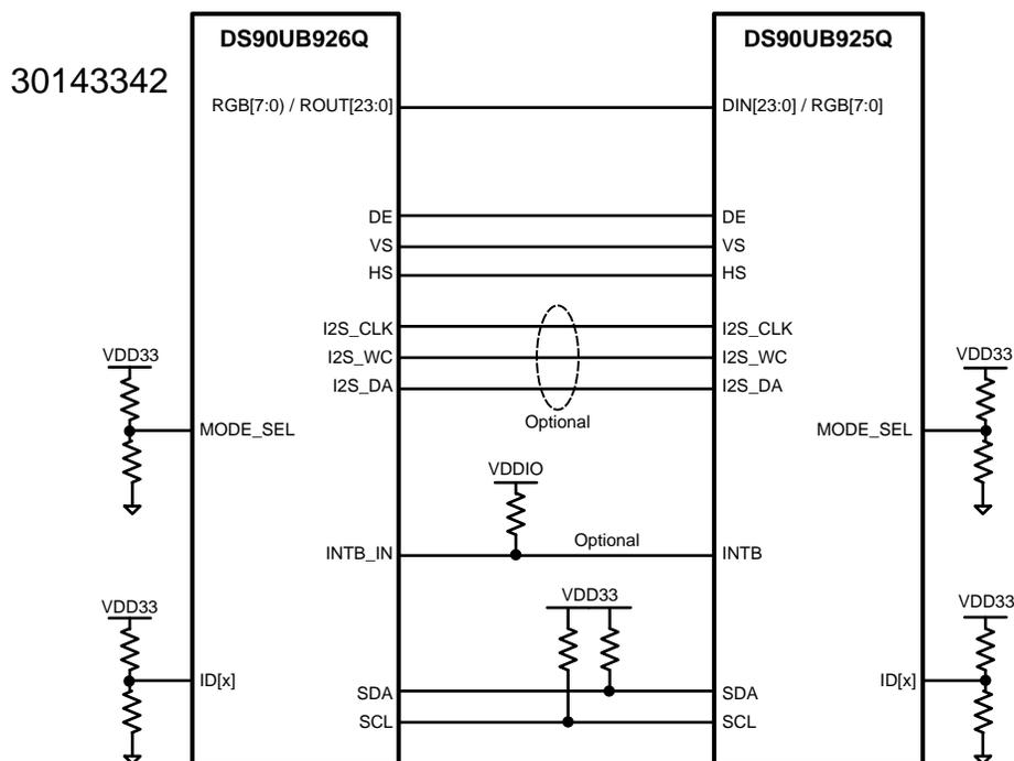
Figure 15. Repeater Connection Diagram
