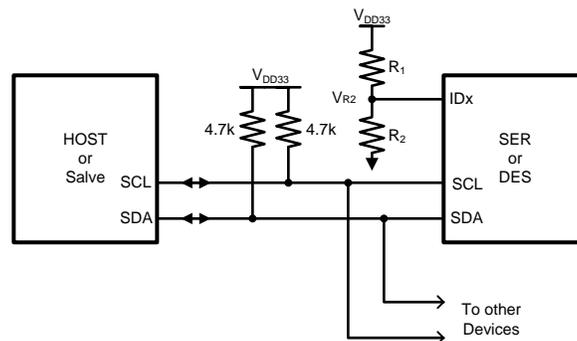
Figure 18. Serial Control Bus Connection
