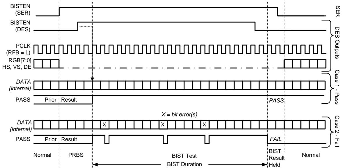
Figure 29. BIST Waveforms
