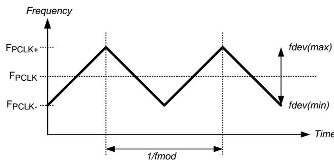
**Figure 22. SSCG Waveform**
