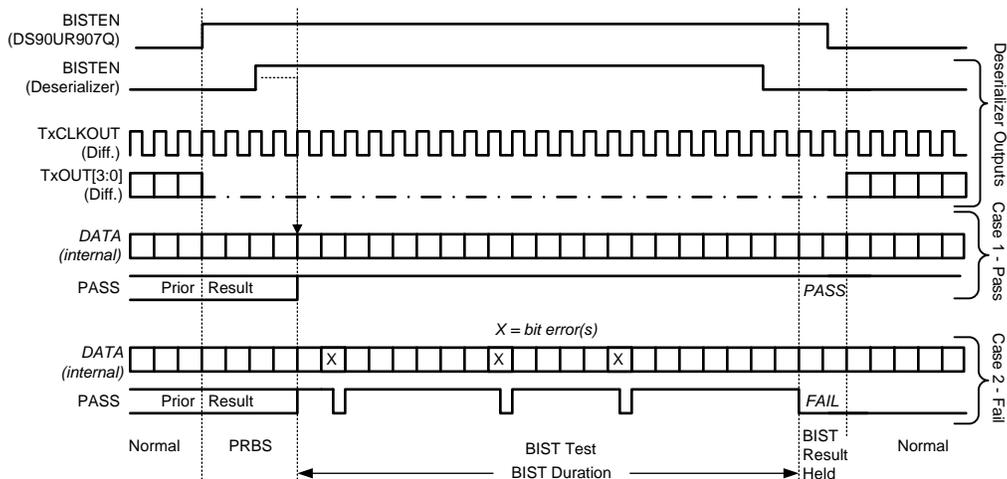
Figure 21. BIST Waveforms
