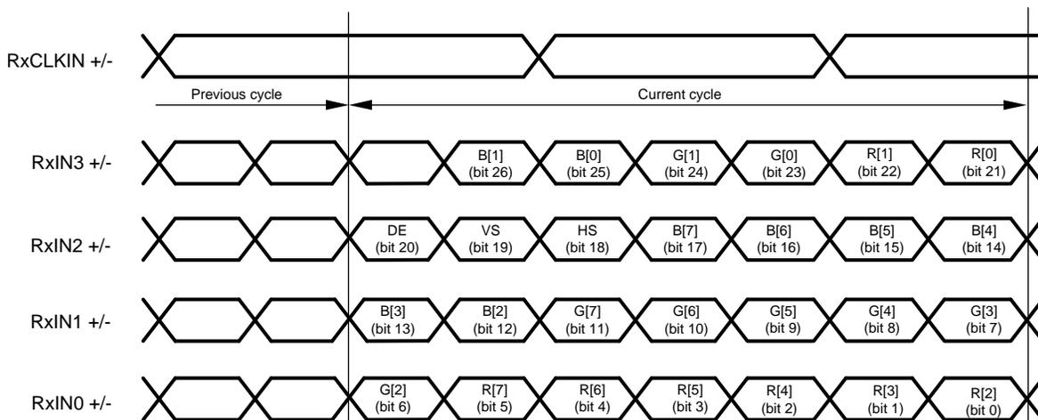
Figure 17. 8-bit FPD-Link Mapping: LSB's on RxIN3
