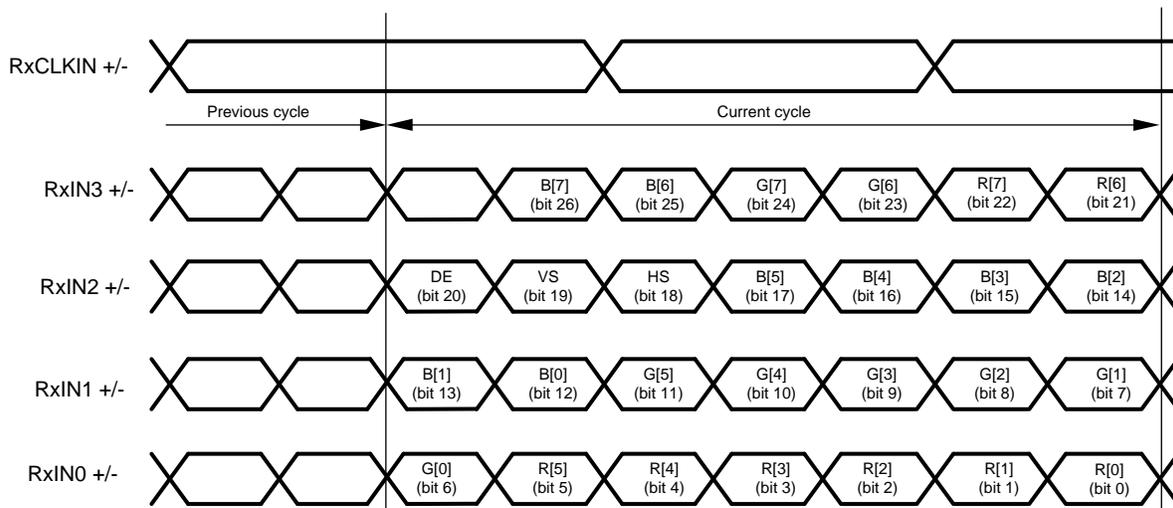
**Figure 18. 8-bit FPD-Link Mapping: MSB's on RxIN3**
