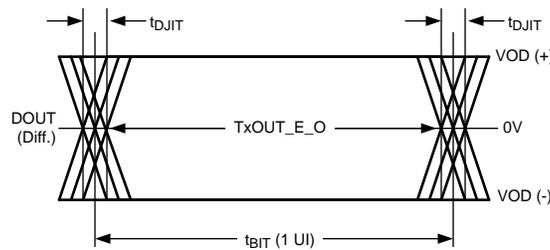
Figure 10. Output Jitter
