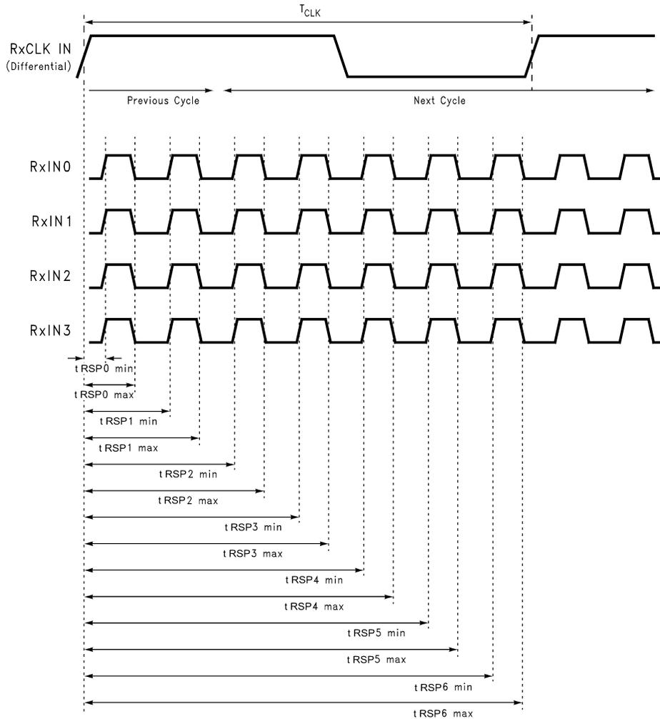
Figure 6. FPD-Link Input Jitter Tolerance
