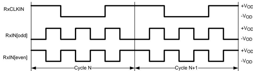
Figure 11. Checkerboard Data Pattern
