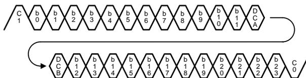
Figure 15. FPD-Link II Serial Stream
