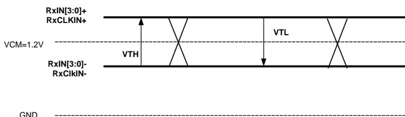
Figure 2. FPD-Link DC VTH/VTL Definition
