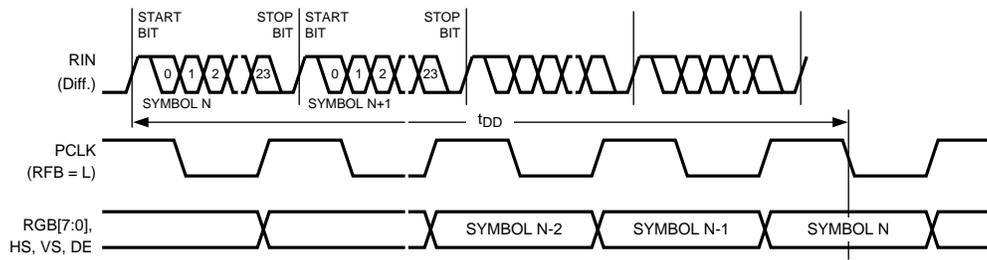
Figure 4. Deserializer Delay – Latency
