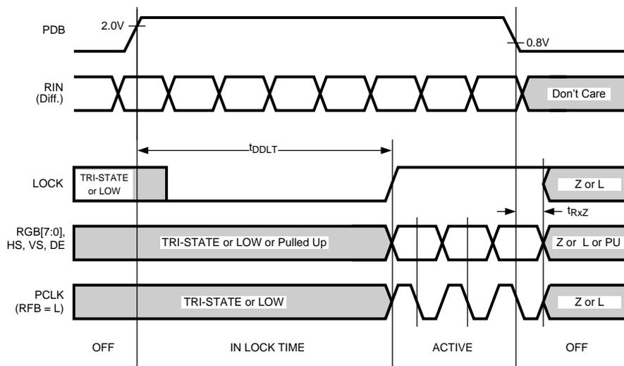
Figure 6. Deserializer PLL Lock Times and PDB TRI-STATE Delay
