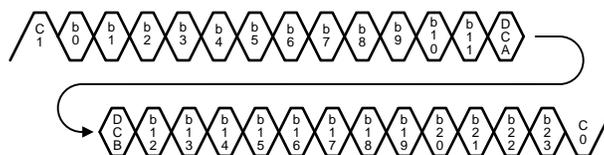
**Figure 12. FPD-Link II Serial Stream (905/916)**
