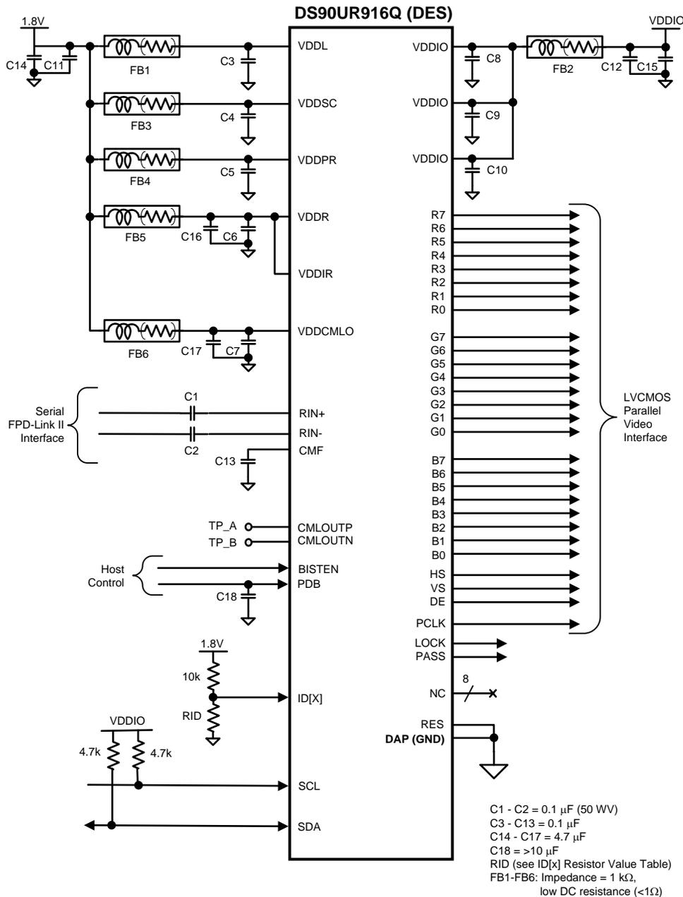
Figure 29. DS90UR916Q Typical Connection Diagram — Pin Control
