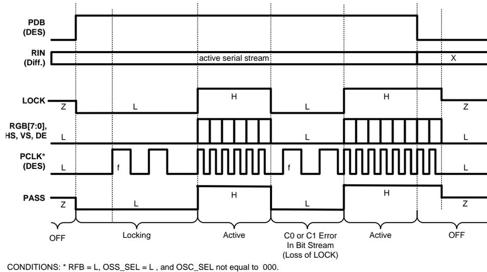
Figure 20. Des Outputs with Output State High and PCLK Output Oscillator Option Enabled
