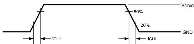
Figure 3. Deserializer LVCMOS Transition Times
