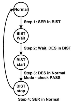
**Figure 23. BIST Mode Flow Diagram**
