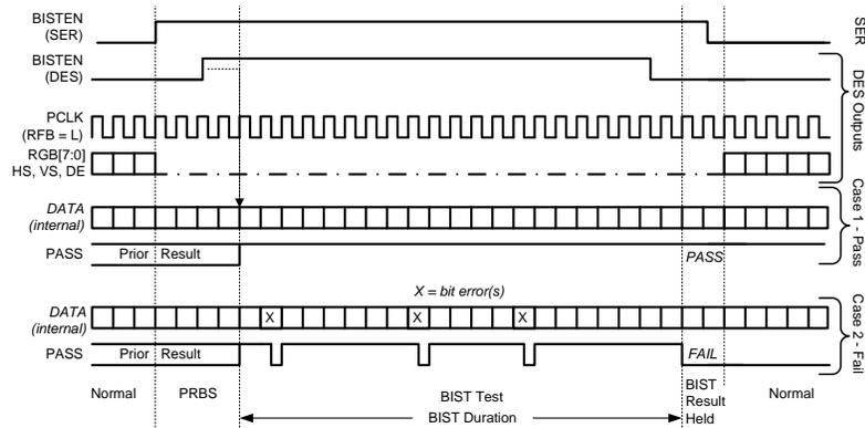
Figure 24. BIST Waveforms
