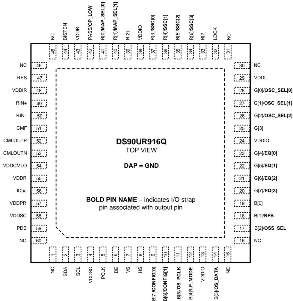
Figure 1. Deserializer - DS90UR916Q — Top View
