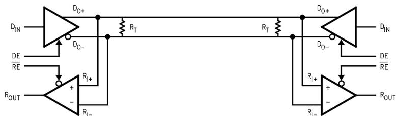
**Figure 12. Bi-Directional Half-Duplex Point-to-Point Applications**
